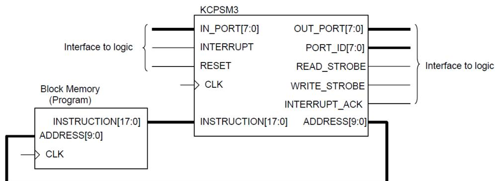
The most important feature of this microcontroller is that it is completely embedded in the FPGA and does not require additional external circuits to operate. Inside the FPGA, it can be connected to any other element that performs advanced logic functions. The KCPSM3 project was written in VHDL. The architecture of the microcontroller is shown in the block diagram below.
