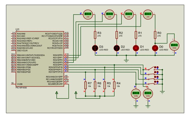
Figure 1. LEDs and switches connected on the same parallel port
